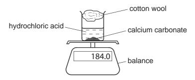
The beaker was placed on a balance and the mass of the beaker and contents recorded every minute.
